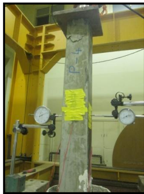
Figure (12) P-4 Flange Buckling
