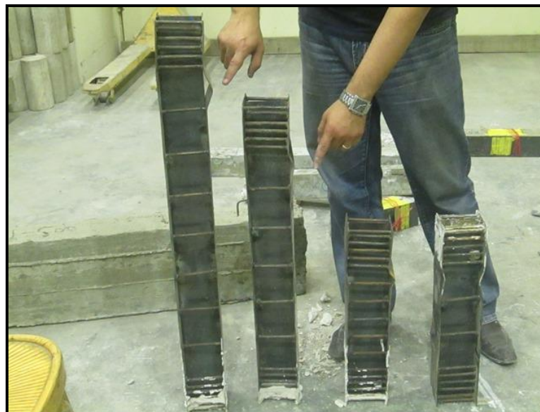
Figure (16) Bare Steel Specimens after Failure
