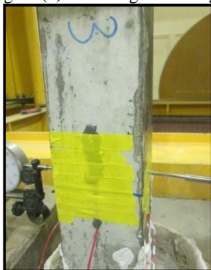
Figure (9) P-3 Flange separation
