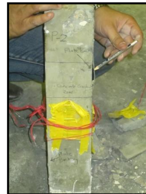
Figure (8) P-2 Failure zones
