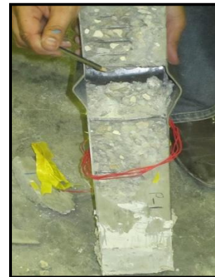
Figure (5) P-1 Web Buckling
