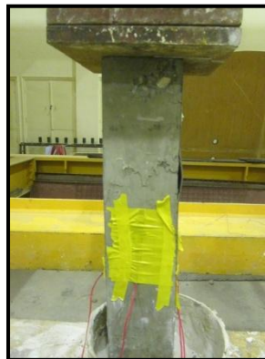
Figure (7) P-2 Concrete Cracks
