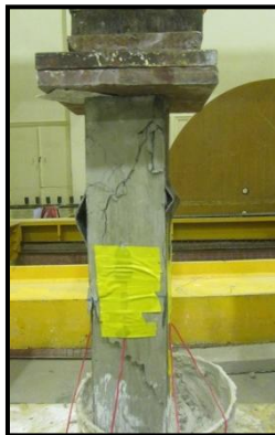
Figure (3) P-1 Flange Bucklin
