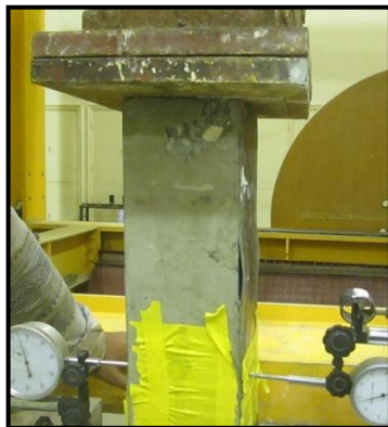
Figure (6) P-2 Flange Buckling
